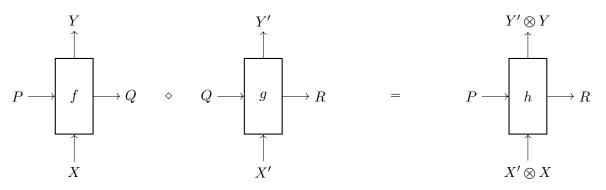
where the horizontal arrows represent the parameters and the vertical arrows the inputs and outputs.
