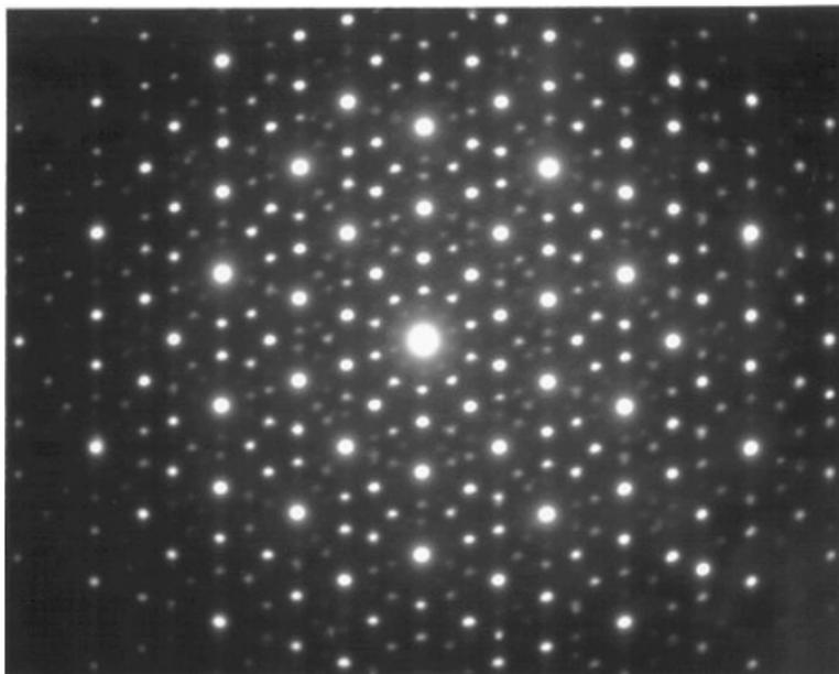
Rapidly cooled alloy of Al with a 10-fold symmetric diffractogram.
