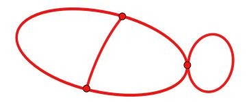
The resulting multigraph is the **core** of the initial graph
