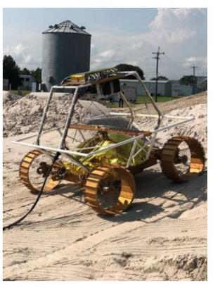
Pictured here is a VIPER mobility testbed, an engineering model created to evaluate the rover's mobility system. The testbed includes mobility units, computing and motor controllers. Testing involves evaluating performance of the rover as it drives over various slopes, textures and soils that simulate the lunar environment.
