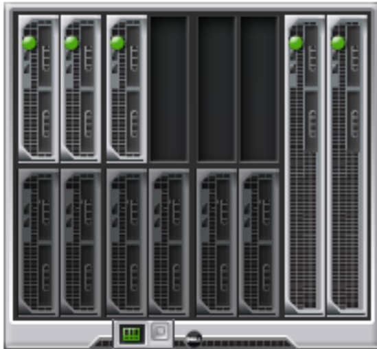
Chassis Dell M1000e 6 x M630 [ 700 Go RAM – 2 x Xeon 2.6 GhZ ] 2 x MXL – 40 G / FCoE
