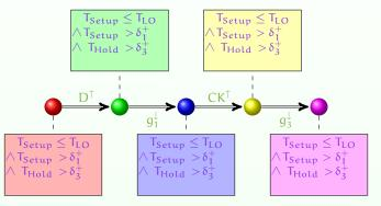
$$\begin{array}{llll} \pi_0: \\ \delta_1^- = 7 & \delta_1^+ = 7 & T_{HI} = 24 \\ \delta_2^- = 5 & \delta_2^+ = 6 & T_{LO} = 15 \\ \delta_3^- = 8 & \delta_3^+ = 10 & T_{setup} = 10 \\ \delta_4^- = 3 & \delta_4^+ = 7 & T_{Hold} = 17 \end{array}$$
