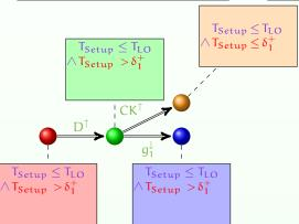
$$\begin{array}{llll} \pi_0: \\ \delta_1^- = 7 & \delta_1^+ = 7 & T_{HI} = 24 \\ \delta_2^- = 5 & \delta_2^+ = 6 & T_{LO} = 15 \\ \delta_3^- = 8 & \delta_3^+ = 10 & T_{Setup} = 10 \\ \delta_4^- = 3 & \delta_4^+ = 7 & T_{Hold} = 17 \end{array}$$
