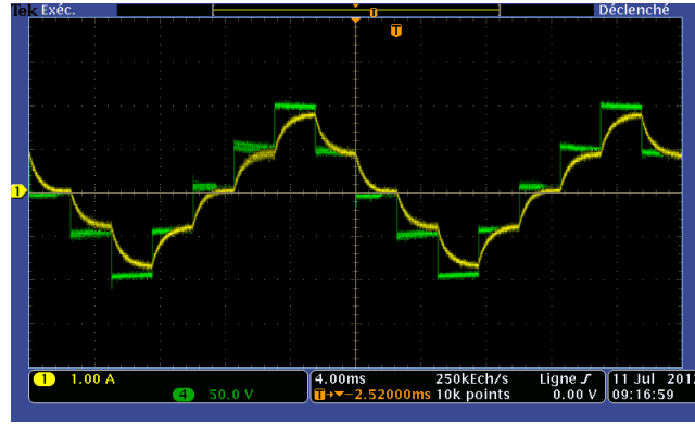
Figure 11: Output voltage (in green) and current (in yellow, after appropriate resizing) in the circuit
