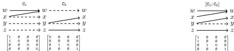
Figure 7: Composition of independent chunks of commands Here C_1 := [w = w + x;] and C_2 := [x = y; z = z * 2] ;
